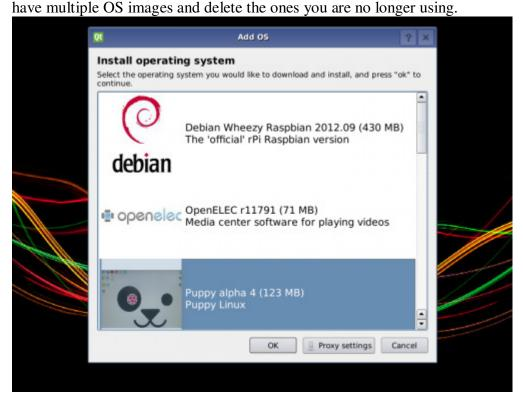
If you are "absolutely" stuck and nothing at all seems to work with your Raspberry Pi system power it down, take the microSDHC card and the SSD out of the Raspberry and plug them into a USB port on your Windows PC. Reformat the microSDHC card to FAT if less than 64Gb and exFAT if more than 64Gb (microSDXC card). If the format worked, it is now blank, copy the Berryboot files back onto it. Reformat the SSD to exFAT because it will be bigger than 64Gb. If the format worked, the SDD is now blank.
